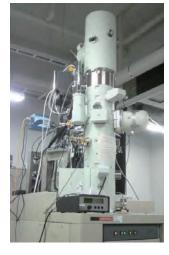
Phase contrast electron cryomicroscope is an electron microscope developed for observing close-to-life state biological samples with a combination of rapid freezing and ice embedding sample preparation methods. Biological specimens up to 200 nm thickness can be observed with high-resolution and high contrast. Structural analyses of protein molecules, viruses, bacteria, cultured cells and frozen tissue sections are performed with this novel microscopic system.
