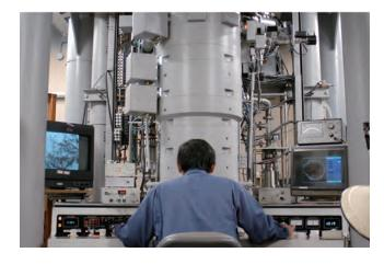
1,000 k. Projections of thick biological specimens up to 5  $\mu$  m are collected at tilt angles between  $\pm$  60° using the side entry specimen holder, which gives 3-dimentional ultra-structures of biological specimens at nanometer scales.
