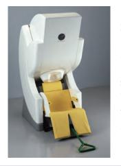
Magnetoencephalography (MEG) has potential to measure brain activities with better temporal and spatial resolution in milliseconds and millimeter, respectively, compared with other methods such as functional magnetic resonance imaging. Event-related magnetic fields following various kinds of sensory stimulation are mainly analyzed. In addition, background brain activities (brain waves) in various conditions can be analyzed.
