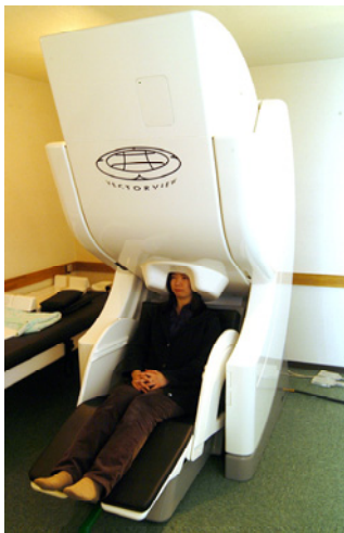
[ELEKTA-Neuromag 社製306 チャンネル脳磁場計測装置] 306-channel helmet-shaped MEG recording system (ELEKTA- Neuromag, Finland)
