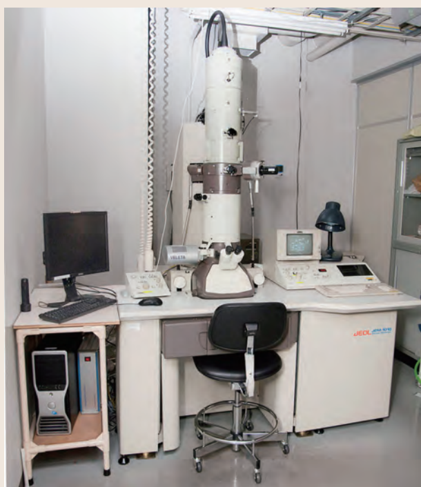
Fig. 2 Transmission electron microscope (TEM) JEOL JEM1010 equipped with 2kx2k CCD camera
