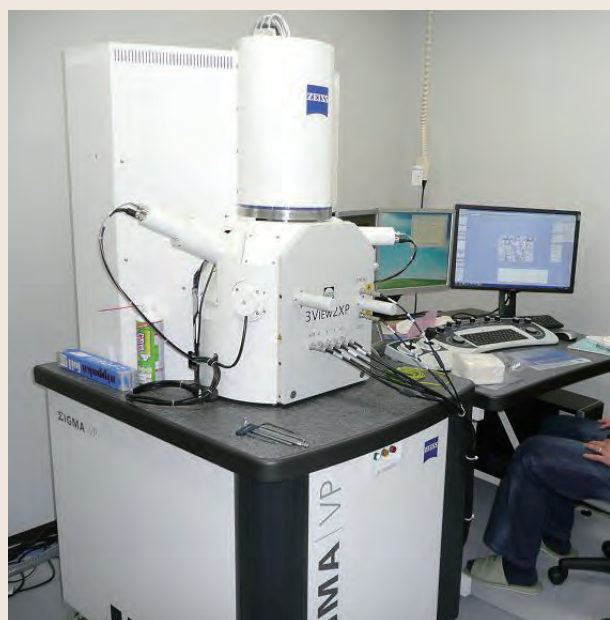
Fig. 1 Serial block-face SEM (SBF-SEM) Gatan 3view - Zeiss \Sigma IGMA/VP
