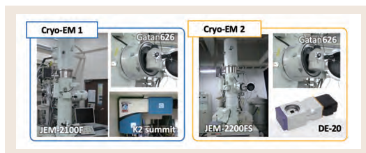
Fig. 1 200kV STEM, JEM2100F with a Gatan K2 camera (left) and 200kV Zernike-phase plate TEM with energy filter and DE-20 camera, JEM2200FS (right). Gatan 626 cryo-transfer holders are used for cryo-EM.
