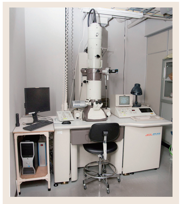
Fig. 2 Transmission electron microscope (TEM) JEOL JEM1010 equipped with 2kx2k CCD camera
