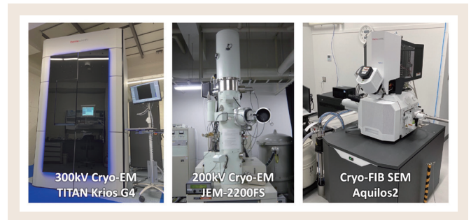
Fig.1 300kV cryo-EM, TITAN Krios G4 (right), 200kV cryo-EM, JEM2200FS (middle), and cryo-FIB SEM (right).
