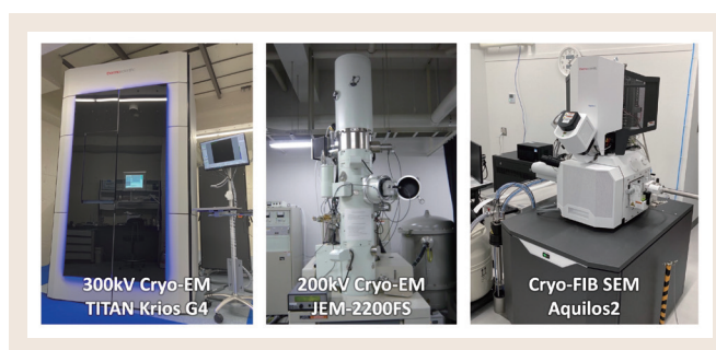
Fig. 1 300kV cryo-EM, TITAN Krios G4 (right), 200kV cryo-EM, JEM2200FS (middle), and cryo-FIB SEM (right).
