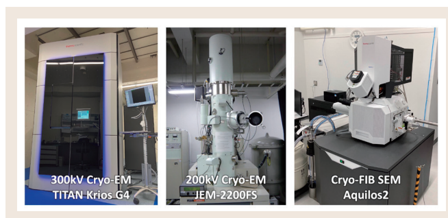
Fig. 1 300 kV cryo-EM, TITAN Krios G4 (right), 200 kV cryo-EM, JEM2200FS (middle), and cryo-FIB SEM, Aquilos2 (right).
