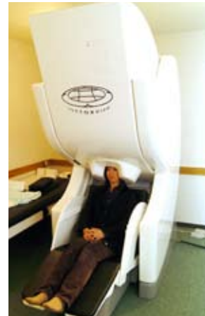
Magnetoencephalography device with 306 channels.
