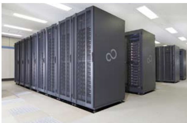
Computer Cluster Fujitsu PRIMERGY RX300S7 Specifications: 126.9TFlops, 5472cores, 342nodes, 43.7TB memory
