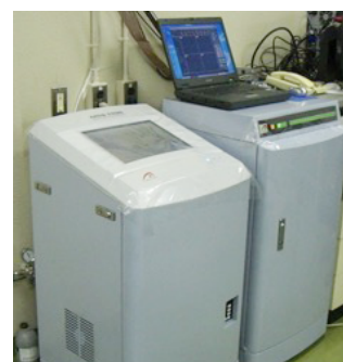
ARCO system: measurement of whole body energy metabolism by mass spectrometrical analysis of respiratory gas exchange
