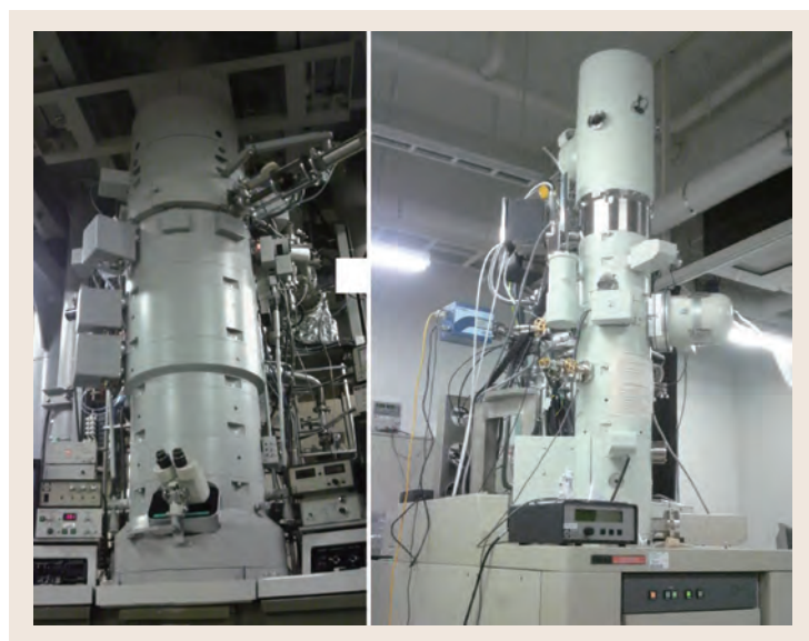
Fig. 1 1M High-voltage electron microscope (HVEM) for biological research, H-1250M (left) and 200kV Phase-contrast cryo electron microscope with energy filter, JEM2200FS (right).
