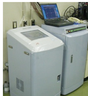
ARCO system: measurement of whole body energy metabolism by mass spectrometrical analysis of respiratory gas exchange
